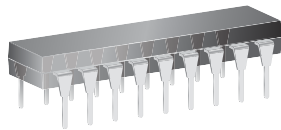
18-pin DIP (A package)
