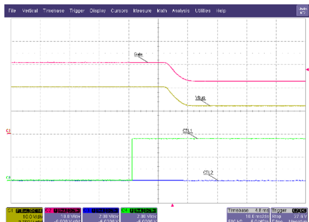
Figure 15. 20-V to 12-V Transition
