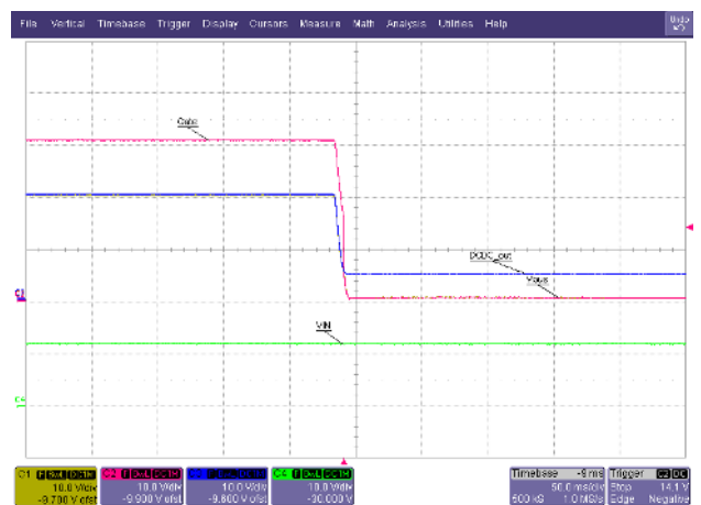
Figure 9. UFP Unplug (20 V)
