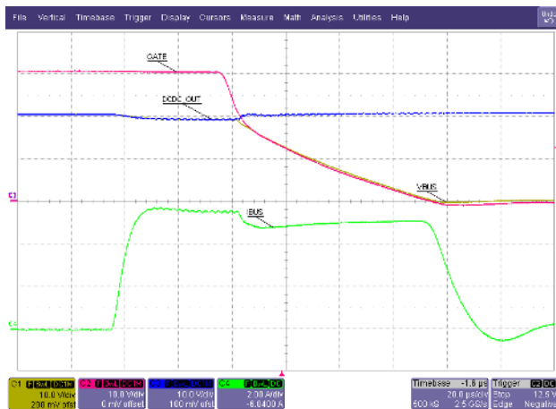
Figure 32. 5.5-A Load Step Triggers OCP (20 V)
