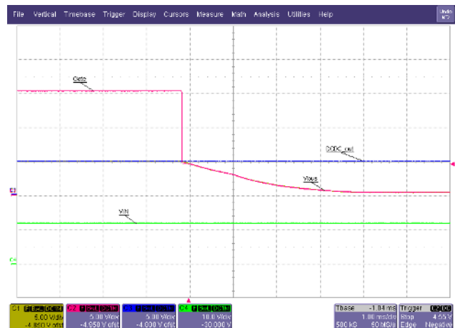
Figure 7. UFP Unplug (5 V)
