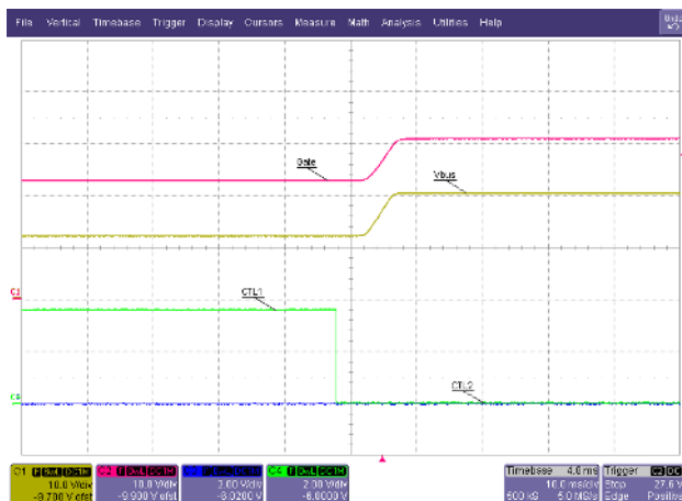
Figure 12. 12-V to 20-V Transition
