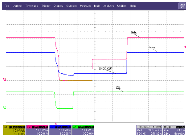
Figure 37. Power Cycle MacBook Plugged In (5-V, 12-V, 20-V Advertised)
