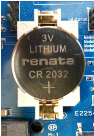
Figure 21: Inserting the coin cell (step 2)
