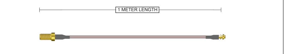
Connector A 132117RP SMA Jack Straight Brass Gold + Heatshrink 50 Ohm RG-316 Continuity/Hi-Pot Connector B 262121 MMCX Jack Straight Bulkhead - Rear Mount Brass Gold + Heatshrink
