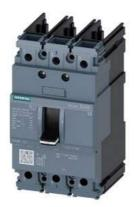
circuit breaker 3VA5 UL frame 125 breaking capacity class S 25kA @ 480V 3-pole, line protection TM210, FTFM, In=90A overload protection Ir=90A fixed short-circuit protection Ii=10 x In UL 489 SB (naval),  $50^\circ$  C without connection
