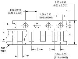
NOTES: TAPE MATERIAL IS PAPER. TAPE THICKNESS IS  $\frac{0.48 \pm 0.03}{(0.019 \pm 0.0012)}$ COVER TAPE ADHESION IS 40 ± 15 GRAMS.
