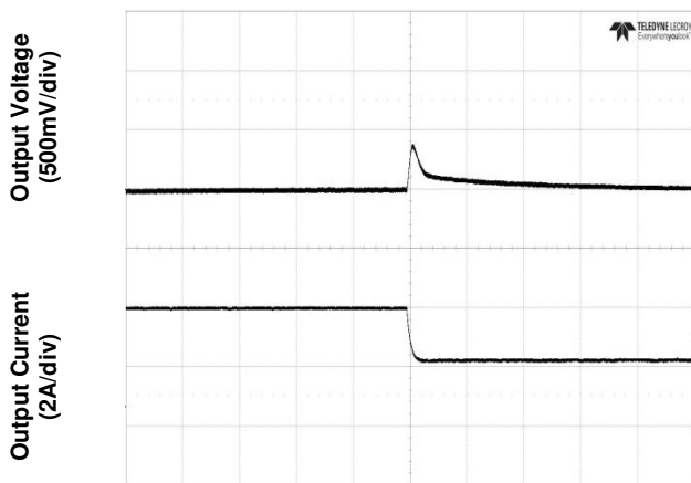
Figure 5. Transient Load Response (typical Vin, load current steps from 50% to 25% at a slew rate 0.1A/μs)
