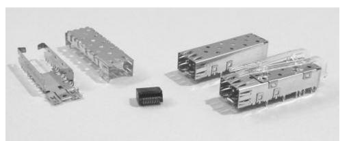
TE offers various termination options for SFP cages, including press-fit, wave solder and IR reflow compatible with tape and reel packaging. The connector is a reliable 20 position interface offered in 0.38 µm (15 µinch) and 0.76 µm (30 µinch) gold plating thicknesses. The connector is packaged in tape and reel for pick and place SMT application. The cage material is a copper alloy with nickel subplate and a matte tin finish.
