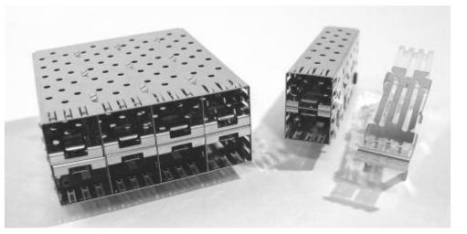
The Stacked SFP product maximizes port density by Taking advantage of the reduced port spacing of the ganged SFP cages, with an added upper port row. The connector is integrated into the cage assembly, using press-fit technology for one-step insertion for cage and connector. Two heights are offered for stacked SFP cages, and available in 2x1, 2x4, and 2x6 port configurations.
