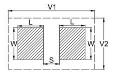
**Density Level A:** For low-density product applications. Recommended for wave solder applications and provides a wider process window for reflow solder processes.
