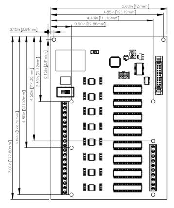
Use the provided spacers and screws when installing the *WaterFeature8*. If other mounting methods are preferred, consider that the board is 0.063" (1.6 mm) thick when selecting mounting devices.
