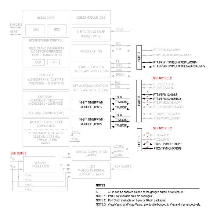
Figure 16-1. MC9S08SG8 Block Diagram with TPM Modules Highlighted
