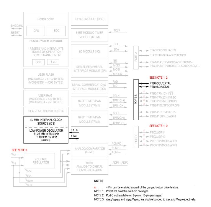
Figure 10-1. MC9S08SG8 Block Diagram with ICS Module Highlighted
