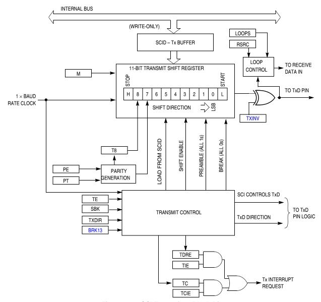
Figure 14-2. SCI Transmitter Block Diagram
