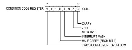
Figure 7-2. Condition Code Register
