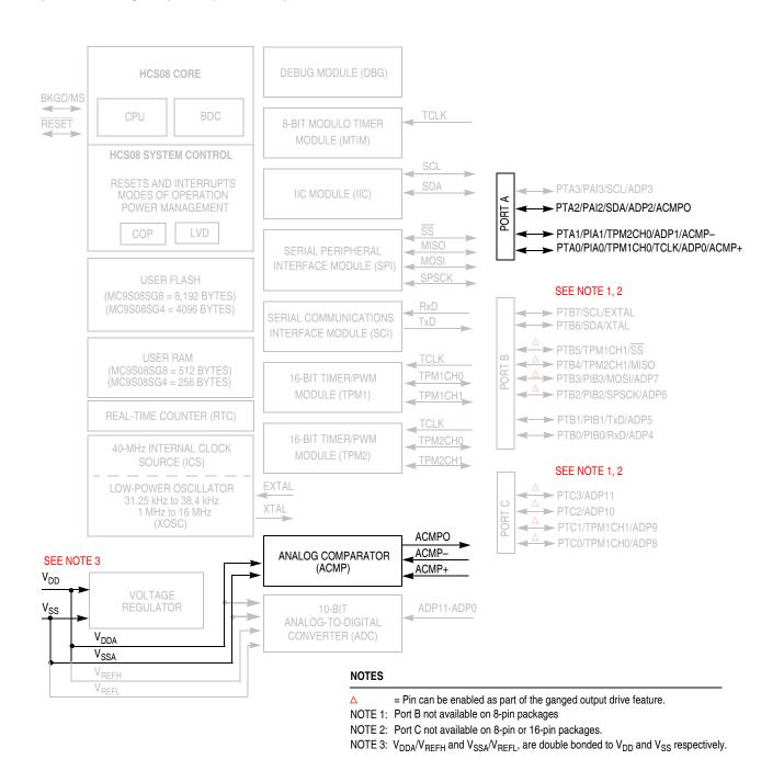
Figure 8-1. MC9S08SG8 Block Diagram with ACMP Module Highlighted
