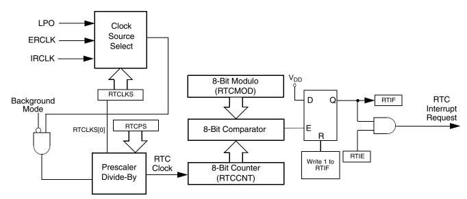
Figure 13-2. Real-Time Counter (RTC) Block Diagram
