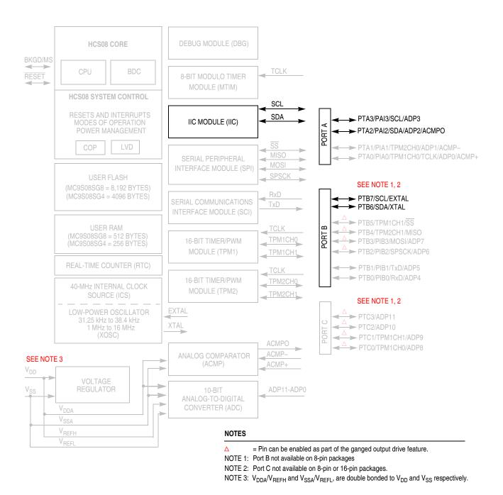
Figure 11-1. MC9S08SG8 Block Diagram with IIC Module Highlighted
