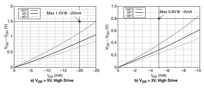
Figure A-3. Typical  $V_{DD}$  –  $V_{OH}$  vs  $I_{OH}$ , High Drive Strength
