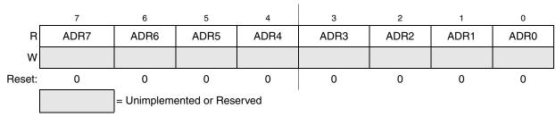
Figure 9-7. Data Result Low Register (ADCRL)
