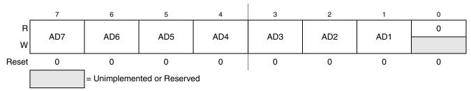
Figure 11-3. IIC Address Register (IICA)
