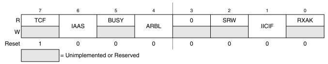
Figure 11-6. IIC Status Register (IICS)
