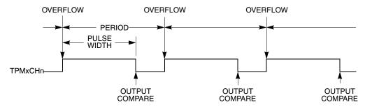
Figure 16-15. PWM Period and Pulse Width (ELSnA=0)
