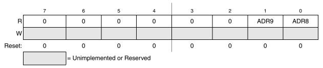
Figure 9-6. Data Result High Register (ADCRH)
