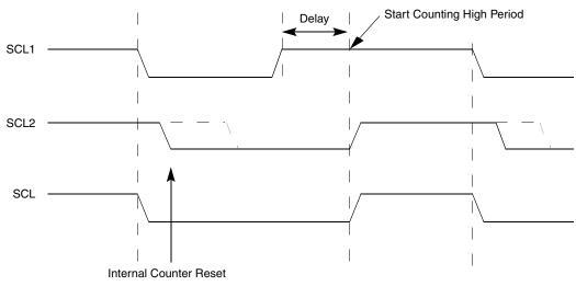
Figure 11-10. IIC Clock Synchronization
