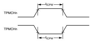
Figure A-13. Timer Input Capture Pulse
