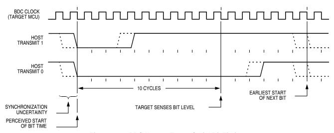
Figure 17-2. BDC Host-to-Target Serial Bit Timing
