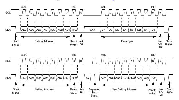
Figure 11-9. IIC Bus Transmission Signals
