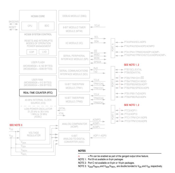
Figure 13-1. MC9S08SG8 Block Diagram with RTC Module Highlighted
