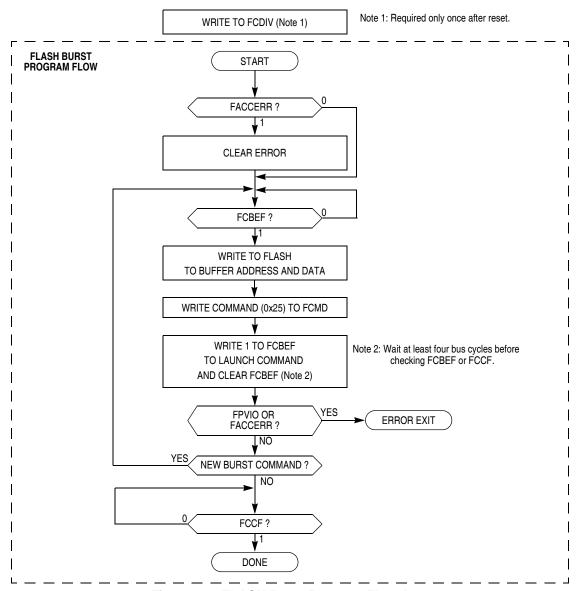
Figure 4-3. FLASH Burst Program Flowchart
