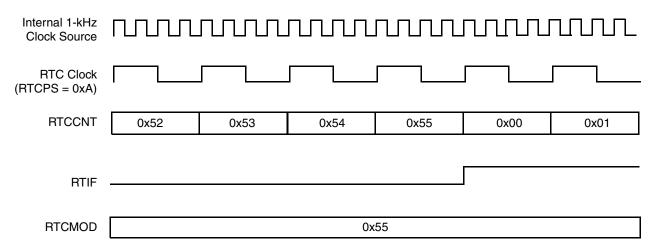
Figure 13-6. RTC Counter Overflow Example
