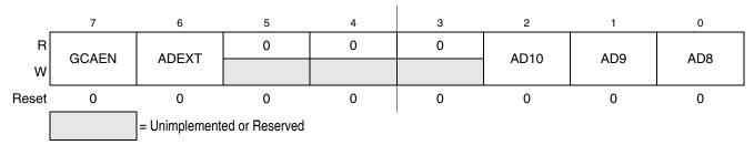
Figure 11-8. IIC Control Register (IICC2)
