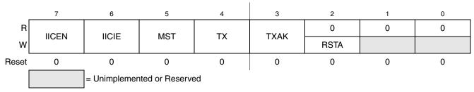
Figure 11-5. IIC Control Register (IICC1)
