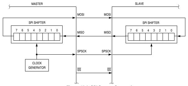
Figure 15-2. SPI System Connections
