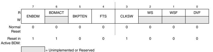
Figure 17-5. BDC Status and Control Register (BDCSCR)
