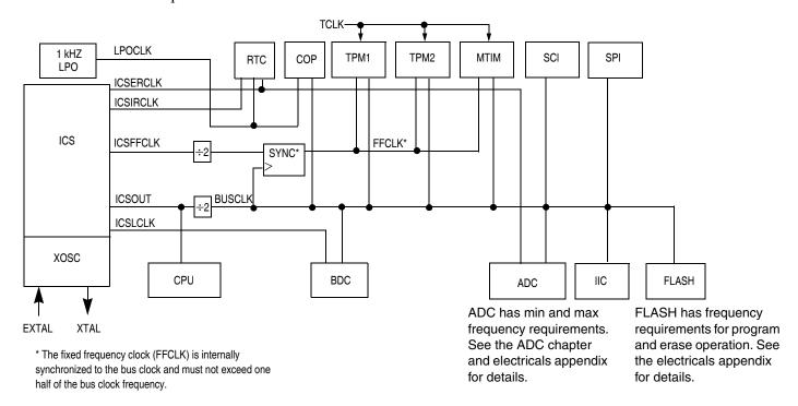
Figure 1-2. System Clock Distribution Diagram
