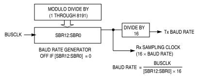
Figure 14-12. SCI Baud Rate Generation
