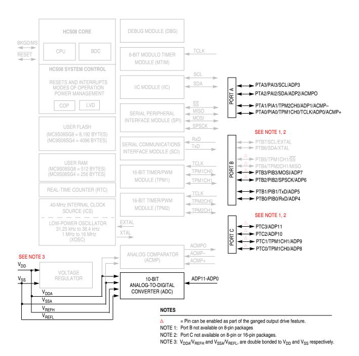
Figure 9-1. MC9S08SG8 Block Diagram with ADC Module Highlighted
