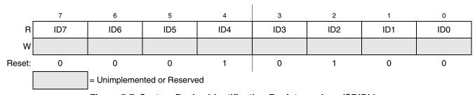
Figure 5-7. System Device Identification Register — Low (SDIDL)
