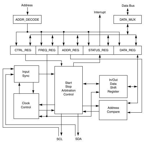
Figure 11-2. IIC Functional Block Diagram
