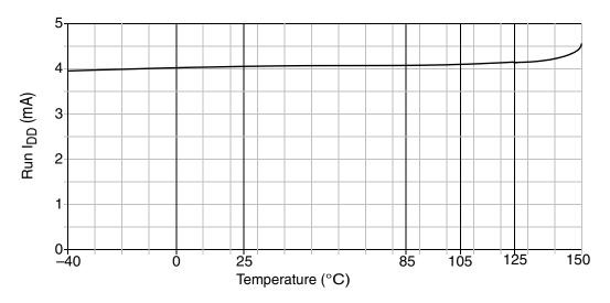
Figure A-6. Typical Run  $I_{DD}$  vs. Temperature ( $V_{DD}$  = 5V;  $f_{bus}$  = 8MHz)
