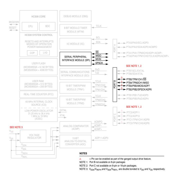
Figure 15-1. MC9S08SG8 Block Diagram with SPI Module Highlighted
