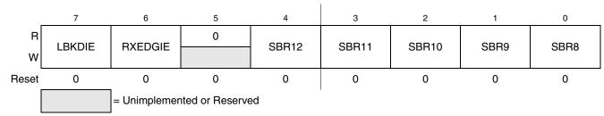
Figure 14-4. SCI Baud Rate Register (SCIBDH)
