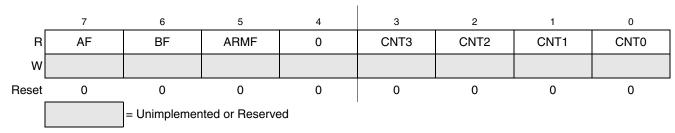
Figure 17-9. Debug Status Register (DBGS)
