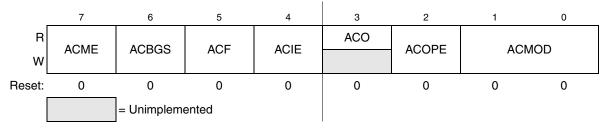
Figure 8-3. ACMP Status and Control Register
