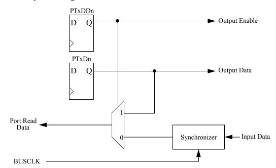
Figure 6-1. Parallel I/O Block Diagram
