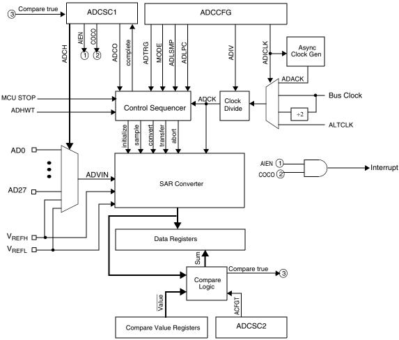
Figure 9-2. ADC Block Diagram
