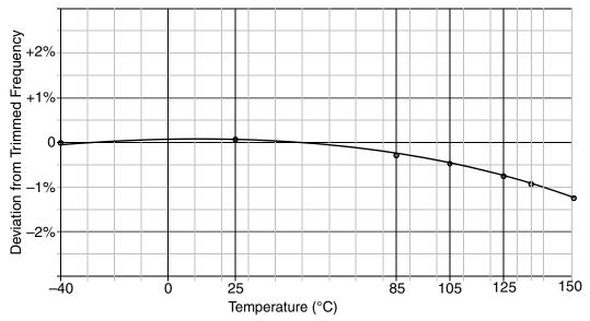
Figure A-8. Typical Frequency Deviation vs Temperature (ICS Trimmed to 16MHz bus@25°C, 5V, FEI)<sup>1</sup>
