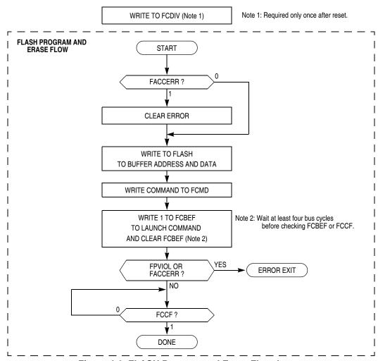
Figure 4-2. FLASH Program and Erase Flowchart
