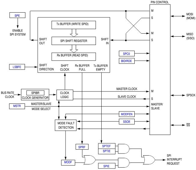
Figure 15-3. SPI Module Block Diagram
