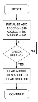
Figure 9-14. Initialization Flowchart for Example
