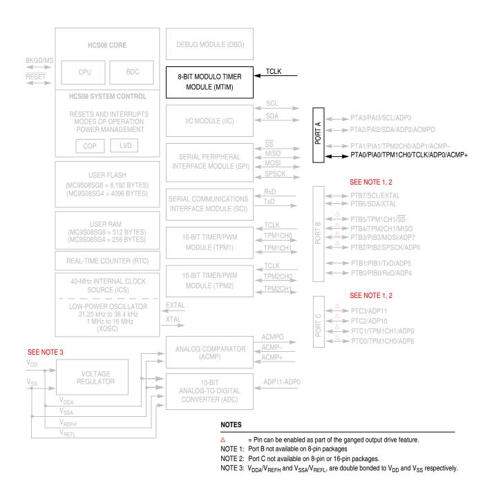
Figure 12-1. MC9S08SG8 Block Diagram with MTIM Module Highlighted
