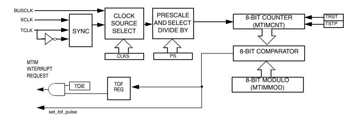
Figure 12-2. Modulo Timer (MTIM) Block Diagram
