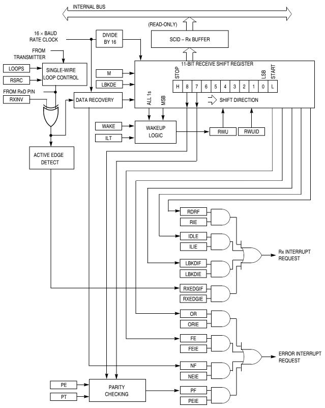
Figure 14-3. SCI Receiver Block Diagram
