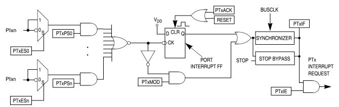
Figure 6-2. Pin Interrupt Block Diagram
