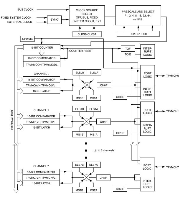
Figure 16-2. TPM Block Diagram
