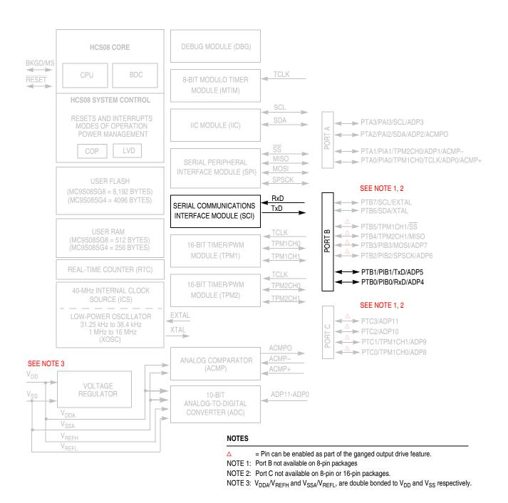
Figure 14-1. MC9S08SG8 Block Diagram with SCI Module Highlighted
