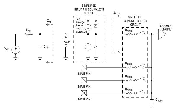
Figure A-9. ADC Input Impedance Equivalency Diagram
