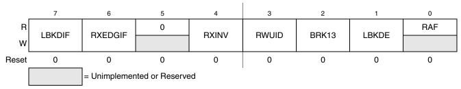
Figure 14-9. SCI Status Register 2 (SCIS2)
