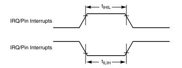
Figure A-11. IRQ/Pin Interrupt Timing
