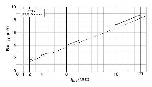
Figure A-5. Typical Run  $I_{DD}$  vs. Bus Frequency ( $V_{DD} = 5V$ )
