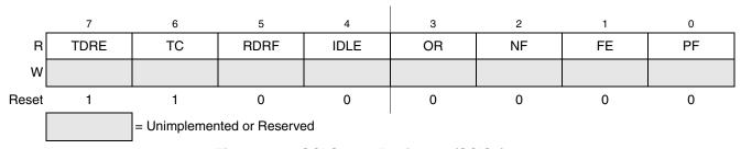
Figure 14-8. SCI Status Register 1 (SCIS1)
