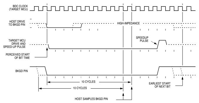
Figure 17-4. BDM Target-to-Host Serial Bit Timing (Logic 0)
