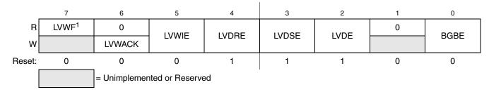
$<sup>^{1}</sup>$  LVWF will be set in the case when  $V_{Supply}$  transitions below the trip point or after reset and  $V_{Supply}$  is already below  $V_{LVW}$
