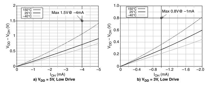
Figure A-4. Typical  $V_{DD} - V_{OH}$  vs  $I_{OH}$ , Low Drive Strength
