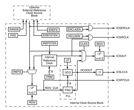
Figure 10-2. Internal Clock Source (ICS) Block Diagram
