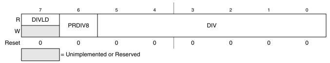
Figure 4-5. FLASH Clock Divider Register (FCDIV)
