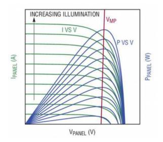
IV/PV characteristic curve of a typical solar panel (picture from Linear Technology)
