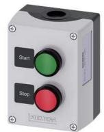
enclosure for command devices, 22 mm, round, enclosure material plastic, enclosure top part gray, 2 control points plastic, B=Pushbutton green, label: start, 1 NO, screw terminal, A=Pushbutton red, label: Stop, 1 NC, screw terminal, floor mounting, 1xM20 each on top and bottom, Labels glued in
