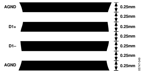
Figure 61. Arrangement of Signal Tracks
