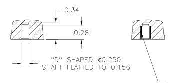
"D" SHAPED SPRING 11125A TO FIT STANDARD Ø0.250 SHAFT FLATTED TO 0.156
