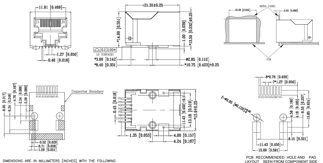
DIMENSIONS ARE IN MILLIMETERS [INCHES] WITH THE FOLLOWING TOLERANCES: [INCHES] ARE FOR REFERENCE ONLY. X.XX=  $\pm 0.25$  [ $\pm .010$ ]
