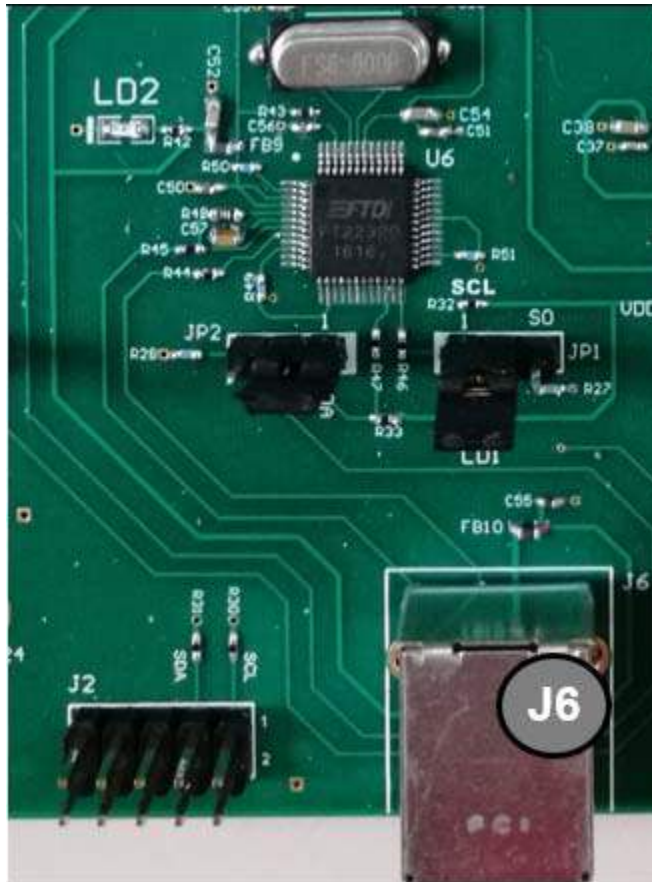
Figure 2. Connecting to a Computer via USB Port J6
