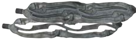
2 Hot forged in the double forging die. The excess burr is removed under an eccentric press.
