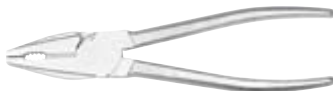
11 Nickel-plated and matt-chrome-plated to prevent dazzle. The electrolytically deposited nickel coating provides the corrosion protection. The electroplated chrome improves the look and gives the pliers a perfect finish.
