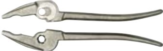
4 The head is machined in a CNC-controlled machining centre. The rivet hole is drilled and counter-bored. The joint clearance and the outer contour are milled. The geometry of the joint area and the coarse and fine toothing are broached.
