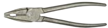
6 The moving and fixed pliers legs are riveted together. A smooth-moving joint with no play is the essential requirement for safe one-handed operation.
