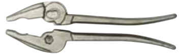
3 The blanks are "normalised" to obtain an even finer-grain, more uniform structure with optimum strength. After descaling, the blanks are calibrated for the following work steps.
