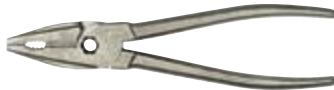
5 The joint faces are precision milled. The pliers head takes on its final form.
