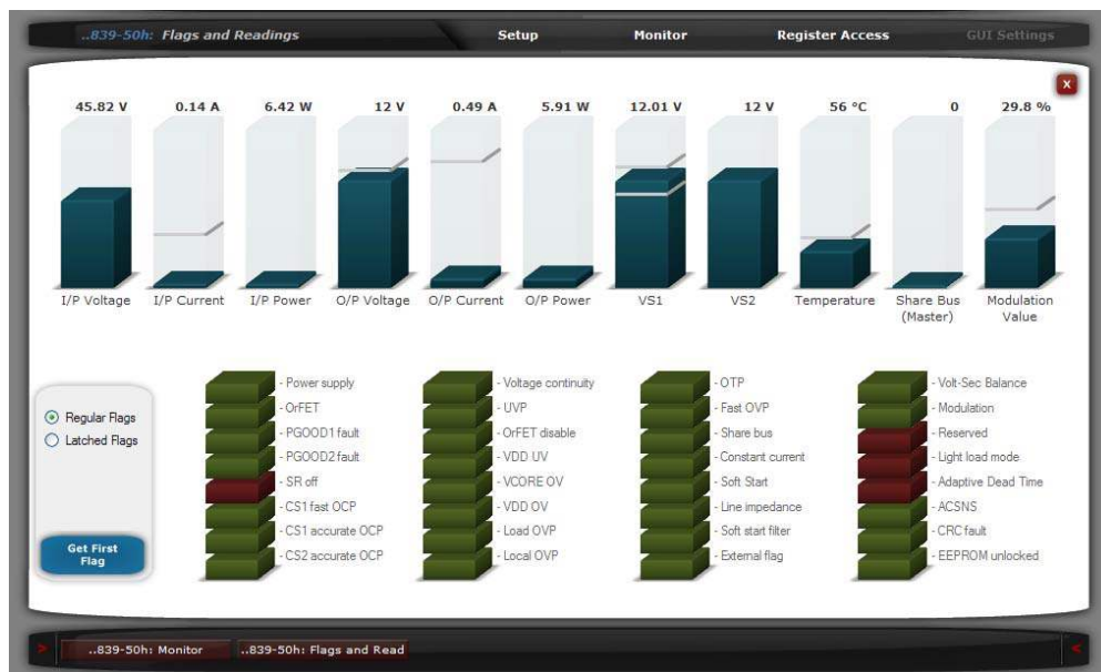
Figure 33 - ACSNS flag tripped during light load mode
