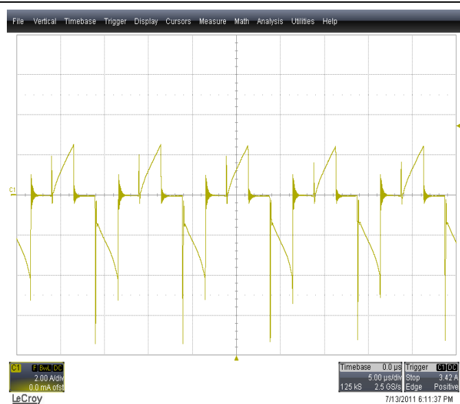
Figure 25 - Primary current with programmed imbalance between PWMs (less than 180 \mu s), 8A load
