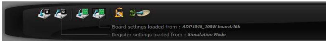
Figure 9 - Different icons on dashboard for loading and saving .46r and .46b files
