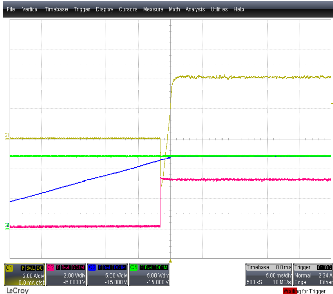
Figure 59 – Output reverse current protection, OrFET enable threshold -384mV Red trace: OrFET gate signal Green and Blue trace: Output voltages of two power supplies Yellow trace: Load current of power supply that is softstarting
