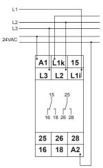
Connected to 1~ 230V mains with power module 230V a.c. without fault latch  $I_{\rm A}{<}10A$
