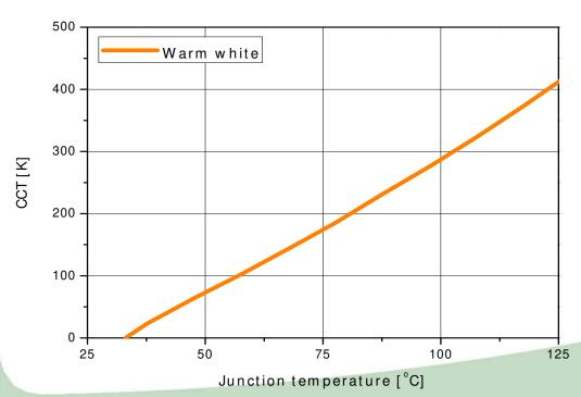
Color coordinate vs. Junction temperature (20mA,RMS@55V,RMS)
