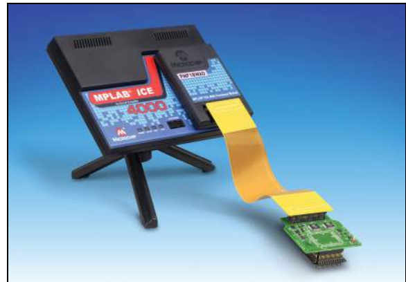
FIGURE 11-5: MPLAB ICE 4000 IN-CIRCUIT EMULATOR
