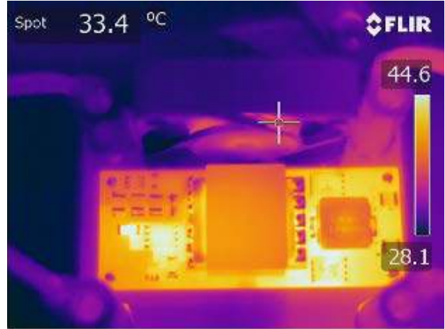
Figure 19. Thermal Image of the ADP1074 with Air Cooling Provided by Fan, 1 Hour Soaking Time
