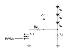
$$\begin{aligned} & \text{MOSFET 'off'} \\ & I_{LED(MIN)} & \frac{V_{FB}}{R_{LED}} \\ & \text{MOSFET 'on'} \\ & I_{LED(MAX)} & \frac{V_{FB}}{R_{LED}} & I_{LED(MIN)} \\ & \text{where V}_{FB} = 100\,\text{mV} \end{aligned}$$
