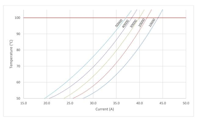
MOSFET Package Temperature for Selected Switching Frequencies in kHz Ambient Temperature 25°C, DC Bus 36V
