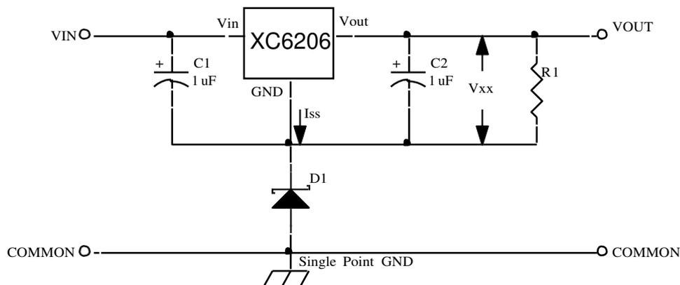
$$V_{out} = V_{xx} + V_{D1}$$
