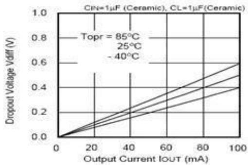
4. Dropout voltage and output voltage
