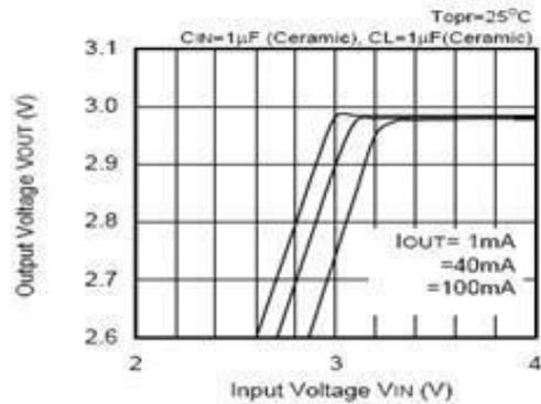
3. Dropout voltage and output current
