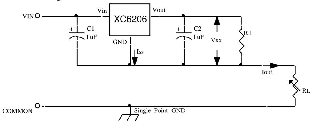
$$I_{out} = V_{xx} / R_A + I_{ss}$$
