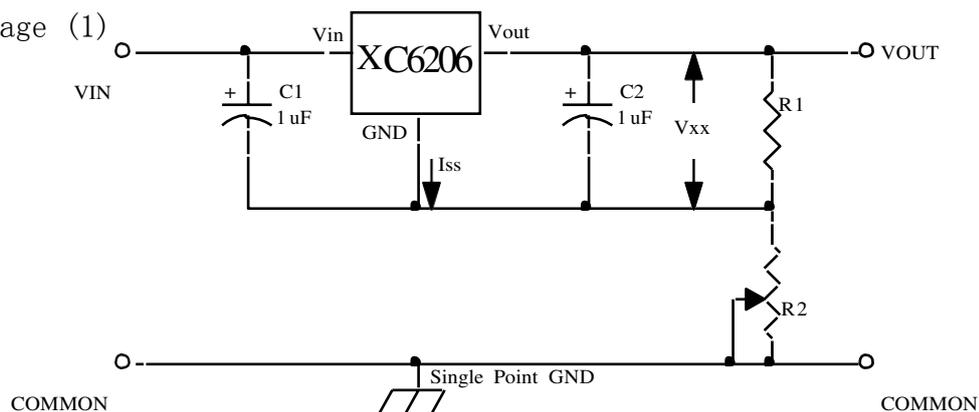
$$V_{out} = V_{xx}(1 + R_2/R_1) + I_{ss}R_2$$
