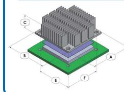
NOTES: 1) Dimension A is the length of the heat sink in the direction of the flow.
