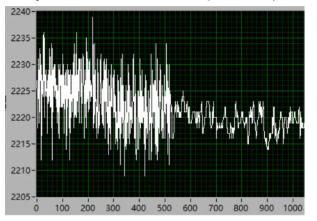
In the figure below, the filter is turned on after 520 points, noise amplitude is 10mm
