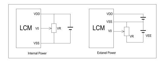
$V_{DD^{\sim}}V_0$ : LCD Driving voltage VR:  $10k^{\sim}20k$
