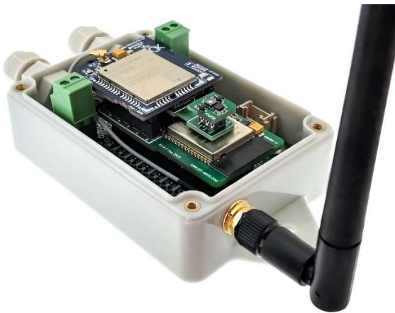
Pic. 20. NB-IOT WiFi / BT / BLE DIY air quality controller
