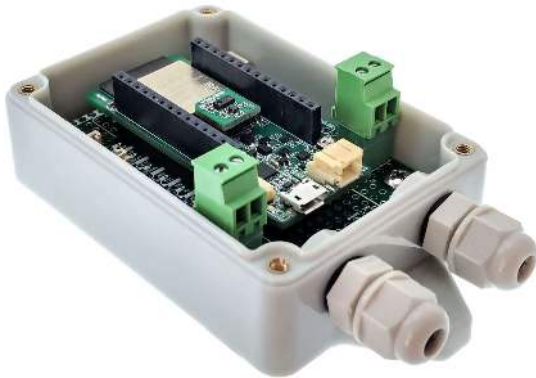
Pic. 22. WiFi ToF sensor : waste collection project
