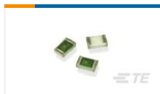
TE Part #1676153-2 RN 0805 10K 0.1% 10PPM 1KRL
