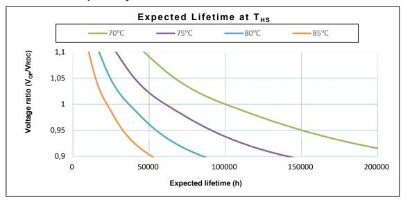
Service life t<sub>LD</sub> at different hotspot temperature (T<sub>hs</sub>) and V<sub>OP</sub>
