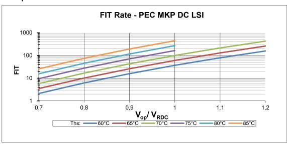
Expected fit rate at different hot spot temperatures (Ths) and voltage VRDC
