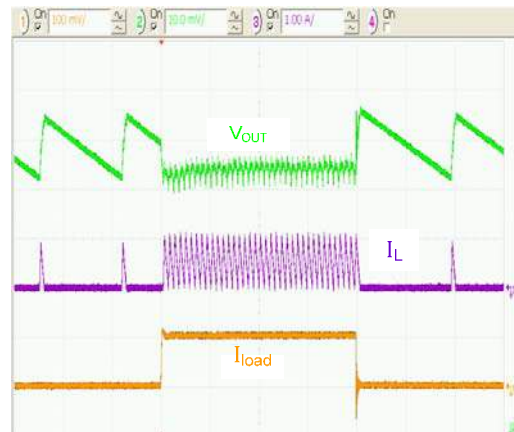
Figure 16. 24 mA to 500 mA to 24 mA, MODE=0, 5 \mu\text{s}/\text{div} .
