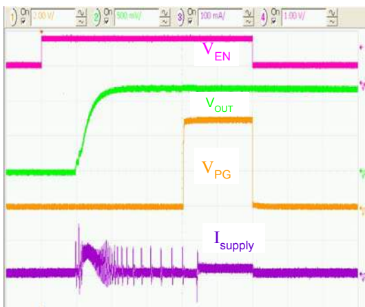
Figure 17. Soft-Start, EN Voltage Raised After V_{IN}=5\text{ V} , I_{LOAD}=0 , 100 \mu\text{s}/\text{div} .
