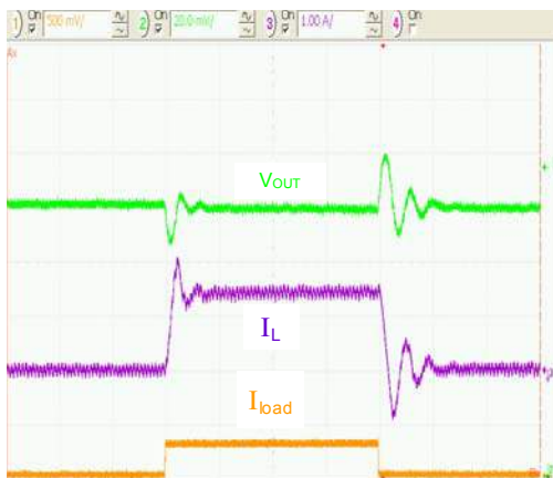
Figure 15. MODE=1, 100 mA to 1.5 A to 100 mA, 5 \mu\text{s}/\text{div} .
