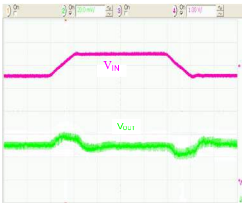
Figure 21. Line Transient Response in PWM Mode, 10\text{ }\mu\text{s/div} .
