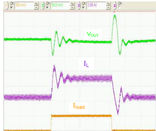
Figure 14. 500 mA to 3 A to 500 mA, 5 \mu\text{s}/\text{div} .
