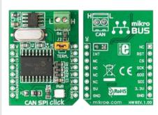
CAN SPI click 5V is an accessory board in **mikroBus**<sup>m</sup> form factor. It is the best solution for adding CAN connectivity to your microcontroller with SPI interface. Board features **MCP2551** CAN transciever circuit which provides CAN serial communication physical layer in accordance with the ISO 11898 standard. It is designed for operation in especially-harsh environments, providing reliable solution. Board is designed to use 5V power supply only.
