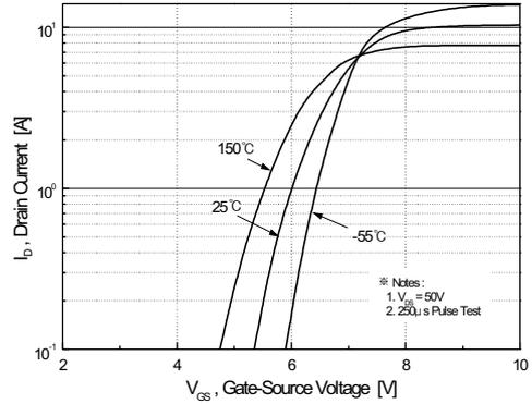
Figure 2. Transfer Characteristics
