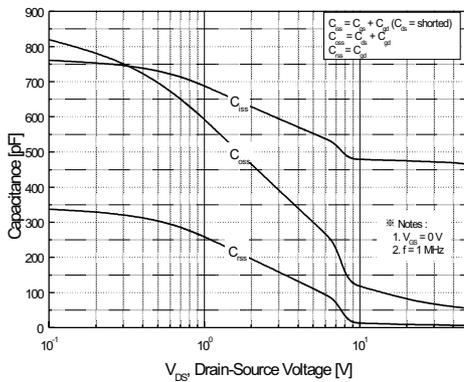
Figure 5. Capacitance Characteristics
