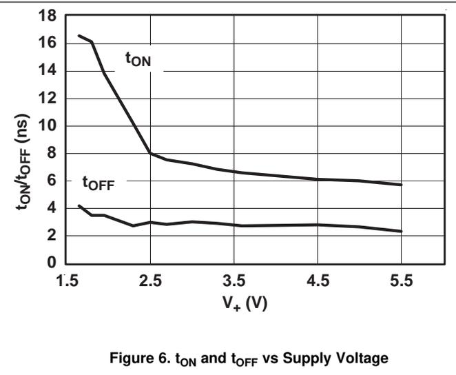
Figure 6.  $t_{ON}$  and  $t_{OFF}$  vs Supply Voltage
