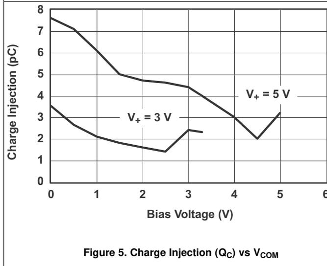
Figure 5. Charge Injection ( $Q_C$ ) vs  $V_{COM}$
