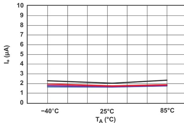
Figure 24. Power-Supply Current vs Temperature
