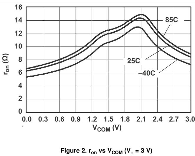
Figure 2.  $r_{on}$  vs  $V_{COM}$  ( $V_+ = 3\text{ V}$ )
