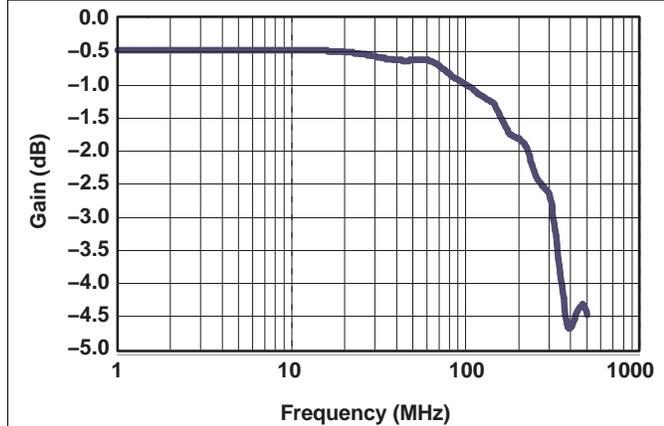
Figure 9. Bandwidth (Gain vs Frequency) (V+ = 5 V)
