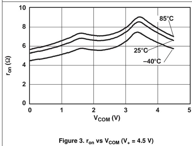
Figure 3.  $r_{on}$  vs  $V_{COM}$  ( $V_+ = 4.5\text{ V}$ )
