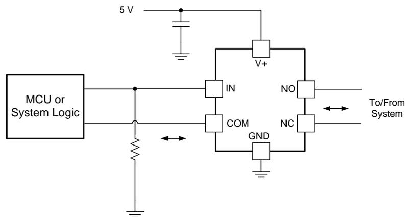
**Figure 23. System Schematic for TS5A3157**
