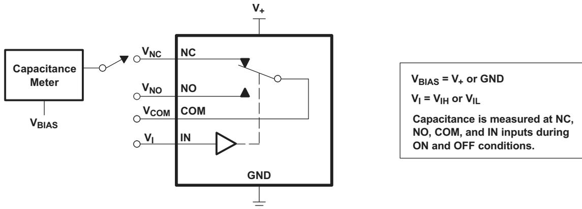
Figure 15. Capacitance ( $C_I$ ,  $C_{COM(ON)}$ ,  $C_{NC(OFF)}$ ,  $C_{NO(OFF)}$ ,  $C_{NC(ON)}$ ,  $C_{NO(ON)}$ )
