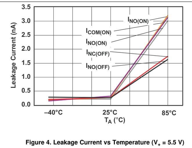
Figure 4. Leakage Current vs Temperature ( $V_+ = 5.5\text{ V}$ )
