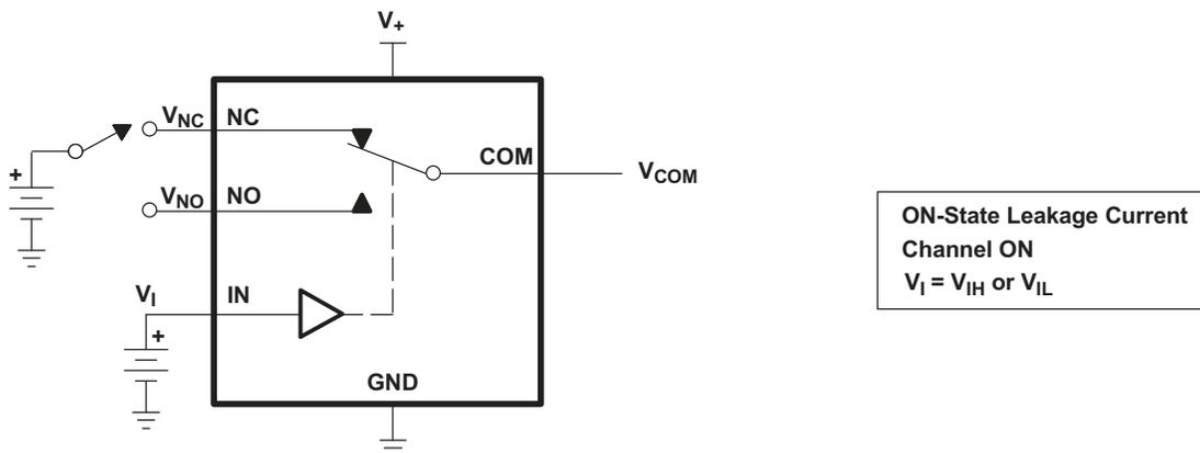
Figure 14. ON-State Leakage Current ( $I_{COM(ON)}$ ,  $I_{NC(ON)}$ ,  $I_{NO(ON)}$ )
