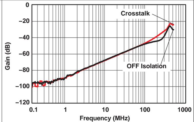
Figure 10. OFF Isolation (V+ = 5 V)
