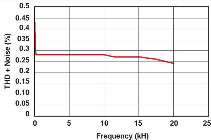
Figure 11. Total Harmonic Distortion vs Frequency
