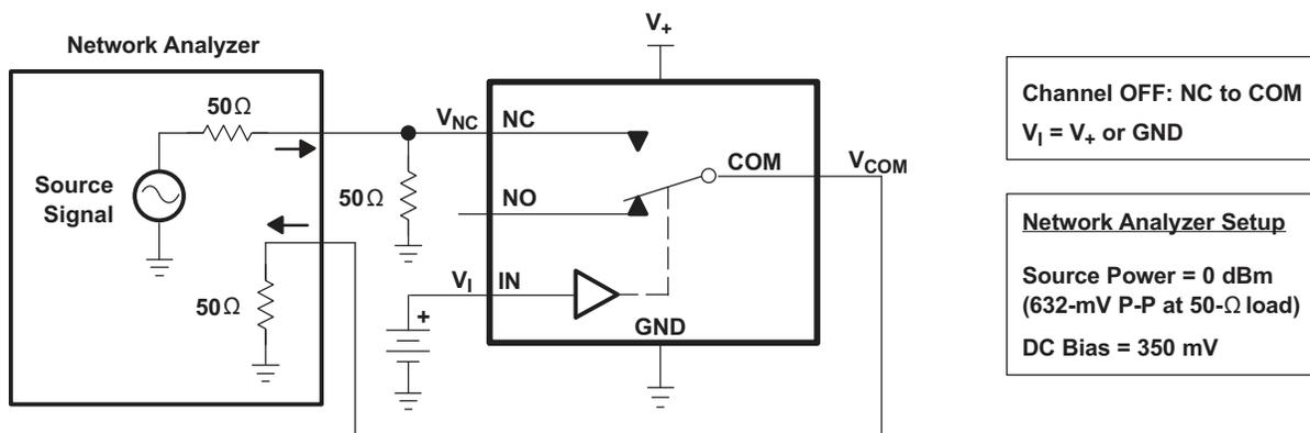
Figure 19. OFF Isolation (O<sub>ISO</sub>)
