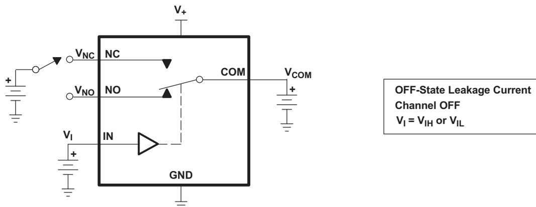
Figure 13. OFF-State Leakage Current ( $I_{NC(OFF)}$ ,  $I_{NO(OFF)}$ )
