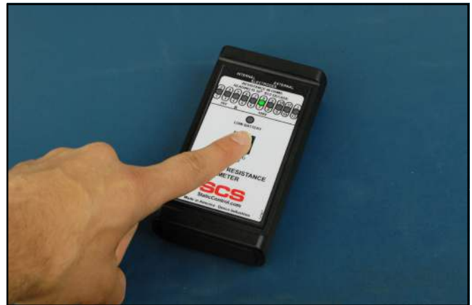
Figure 3. Using the parallel electrodes to measure surface resistance
