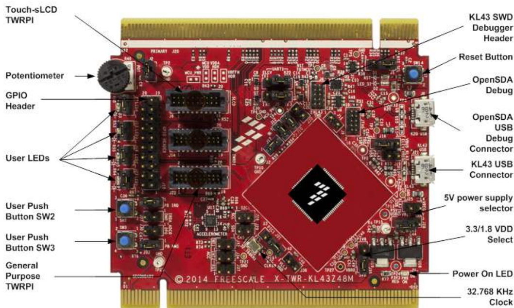
Figure 2. Front side of TWR-KL43Z48M module (TWRPI device not attached)
