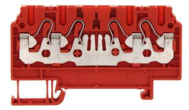
Feed-through terminal, Push-in connection, Mounting type: Mounting rail TS 35/7.5, Rated cross-section: 1.5 mm<sup>2</sup>, Width: 4.1 mm, Colour: Red
