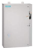
Non-reversing motor starter, Size 3, Three phase full voltage, Solid-state overload relay, OLR amp range 25-100A, 240V 50Hz / 277V 60Hz coil, Combination type, 100A fusible disconnect, 100A/600V fuse clip, Encl NEMA type 4X 304 S-Steel, Water/dust tight noncorrosive, Extra-wide enclosure
