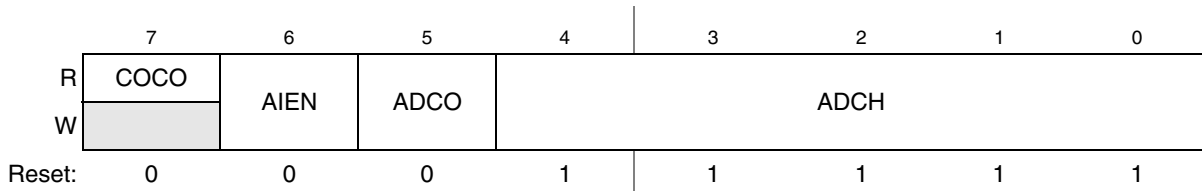
Figure 10-3. Status and Control Register (ADCSC1)
