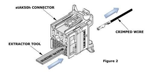
**CAUTION:** This extractor tool should be used to extract the terminal only. Using it for unintended purposes may cause injury or damage to parts. Be careful not to deform the end of the terminal.
