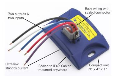
The FlexMod<sup>™</sup> family is a series of small, robust electronic modules. They have two inputs (one analog and one digital) and two solid state outputs (one 10A, one 200mA) that can be programmed to do almost any job.
