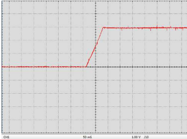
Figure 27. Start-up Waveform at LDA Pin
