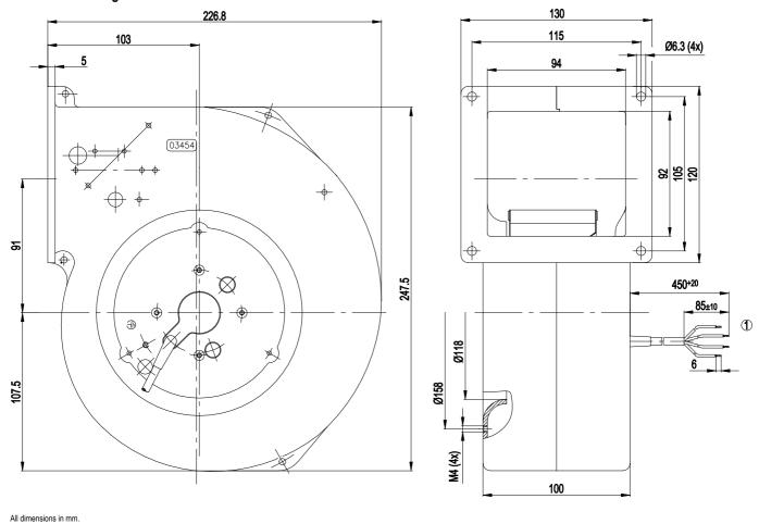
Cable PVC 4G 0.5 mm², 4x crimped splices
