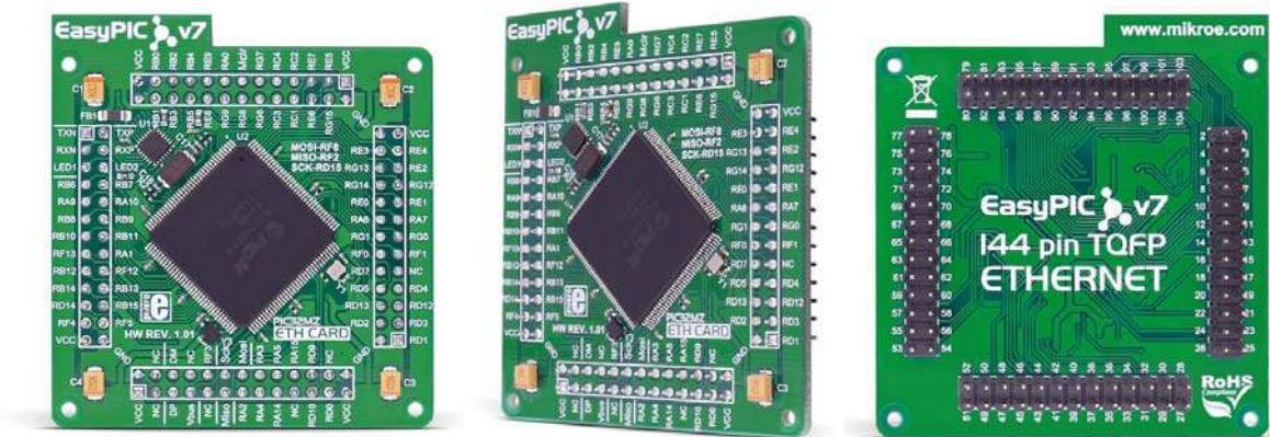
This particular EasyPIC FUSION v7 ETH MCUcard contains the PIC32MZ2048EFH144 microcontroller with on-chip peripherals. It's a great choice for both beginners and professionals. After testing and building the final program, this card can also be taken out of the board socket and used in your final device.
