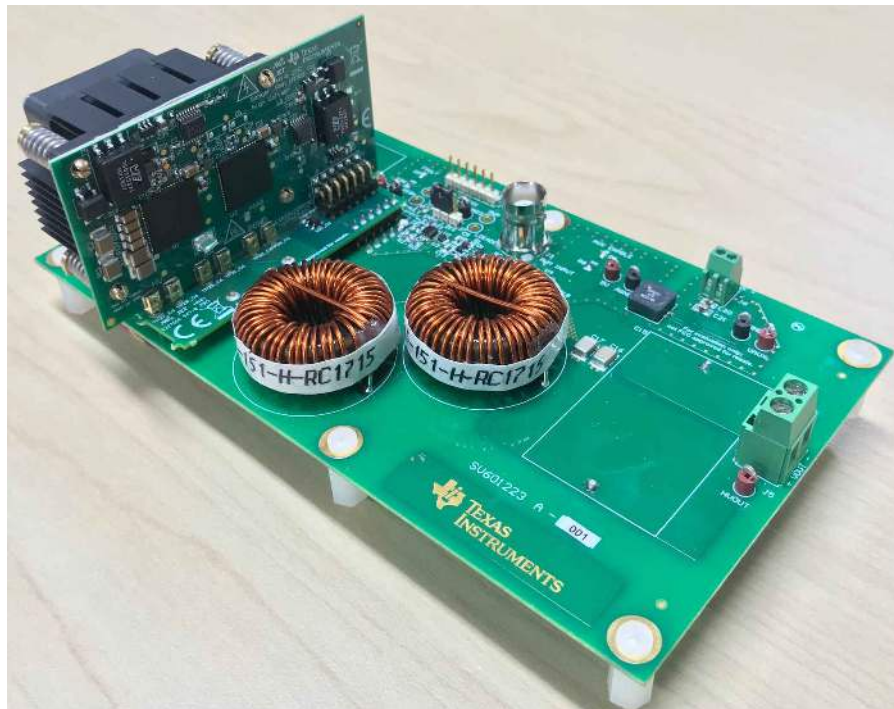
Figure 8-1. LMG342XEVM-04X Connected to the LMG34XX-BB-EVM
