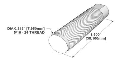
All measurements are in inches [millimeters]
