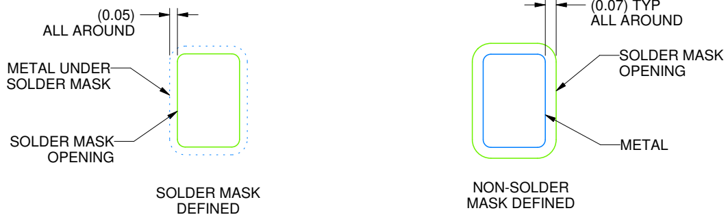
SOLDER MASK DETAIL
