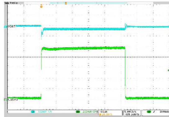
V_{IN} = 12\text{ V} I_O = 5\text{ mA to }1\text{ A to }5\text{ mA} V_{OUT} = 3.3\text{ V} 2.5-MHz Auto T_A = 25^\circ\text{C} PFM/PWM
