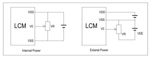
$V_{DD-}V_0$ : LCD Driving voltage VR: 10k~20k
